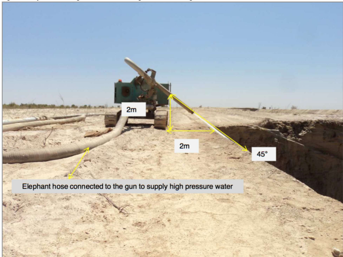
Figure 69: Hydraulic Mining with Monitor showing Distance and Angle
