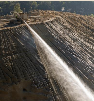
Highly mechanised high-pressure hydro-mining of discarded mine-tailings
