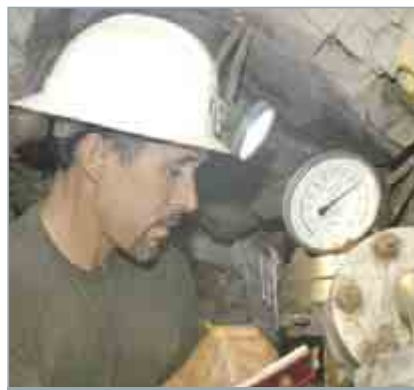
Pumping and plugging: lifelines for ERPM. Shaft foreman Gideon Cramer checks the pressure gauge on the 58 level plug at the mine's Far East Vertical Shaft
